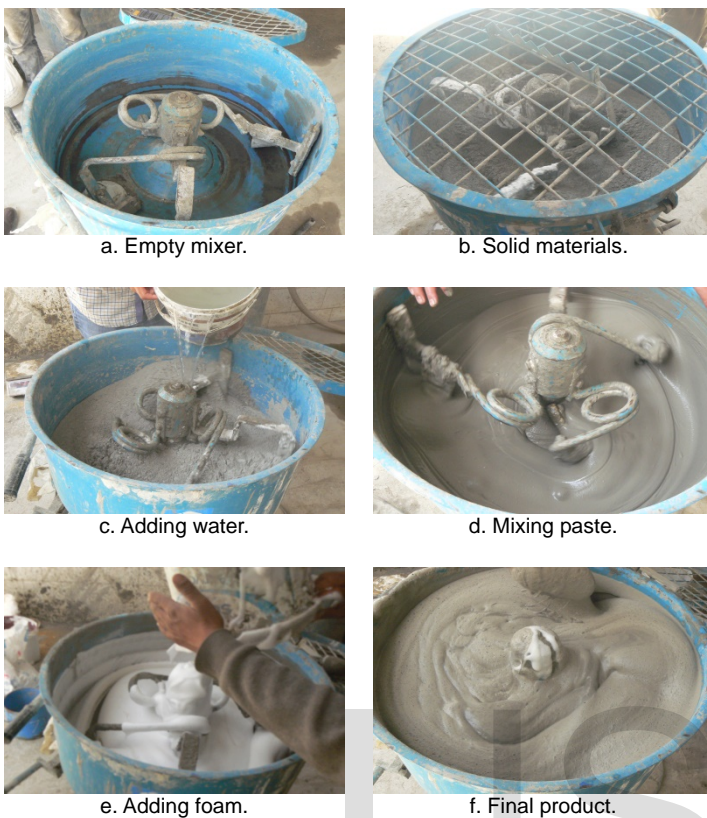
Fig. 3. Foamed concrete manufacturing process.
